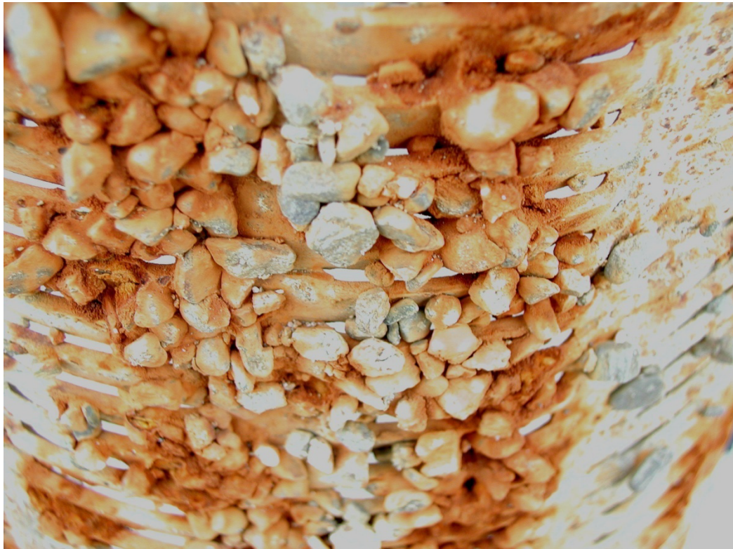
Photo A4.3 – Encrusted Screen Aquifer Side
