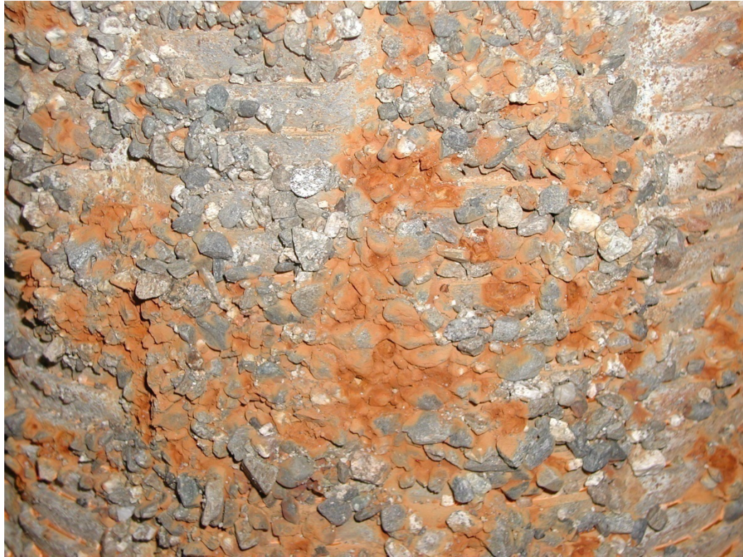
Photo A4.3 – Encrusted Screen Aquifer Side
