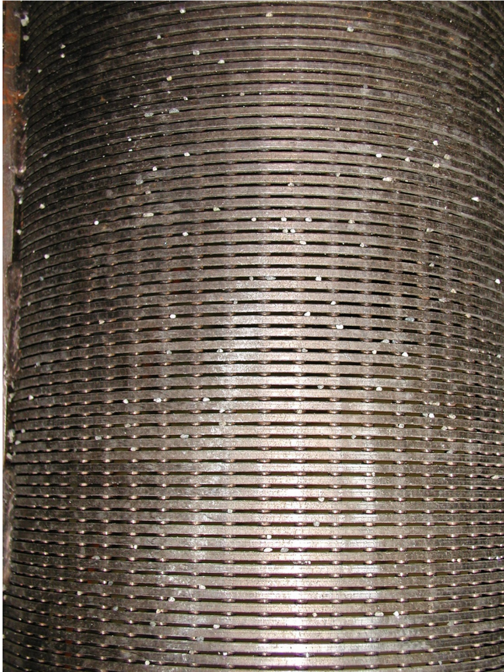
Photo A3.6 – 0.060 SSWWS After Testing
