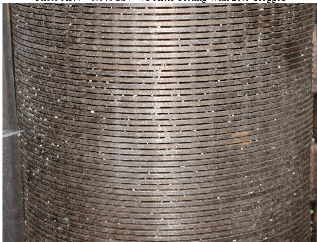
Photo A3.4 – 0.040 SSWWS After Testing With 20% Clogged
