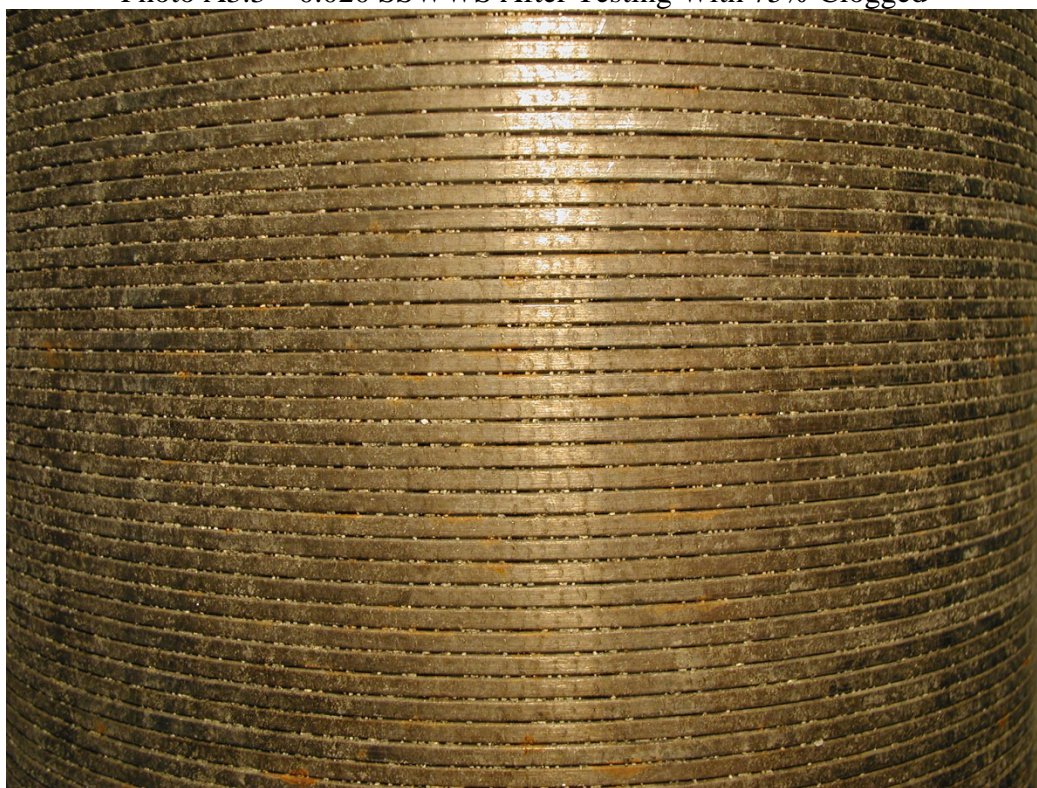
Photo A3.3 – 0.020 SSWWS After Testing With 75% Clogged
