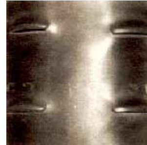
Screen formed by perforating casing in
