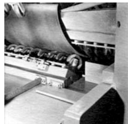
Spiral cylinder forming operation
