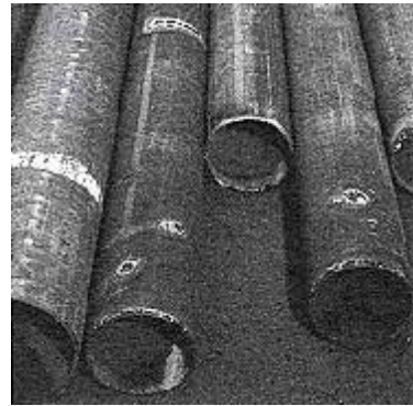
Substandard pipe manufactured from laminated steel has substantially reduced collapsing strength.
