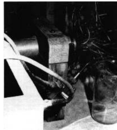
Scanivalve used to record pressures
