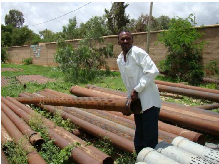
Fig. 2 – Left over, rusted, thin-walled, saw-cut pipe
